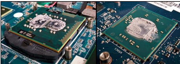
Fig. 4 : Examples for ICs on a notebook mainboard connected to the mainboard via PGA fitted into a socket (left) and directly soldered onto the mainboard (right)
