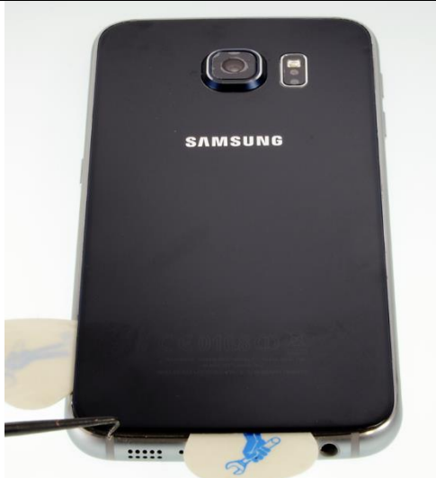
Type A example 3: Separating back cover by dissolving adhesive via thermal energy and carefully prying open the phone
