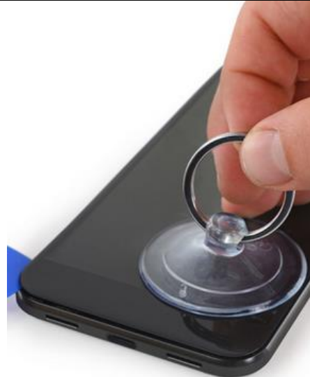
Type B step 3: Separating display unit by dissolving adhesive via thermal energy 1
