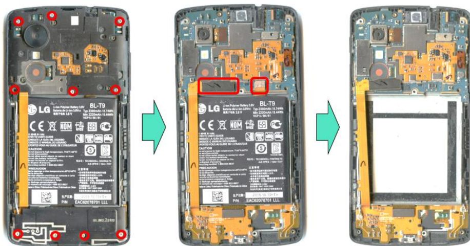
Figure 4: Typical internal designs found in smartphones after removing the back cover.
