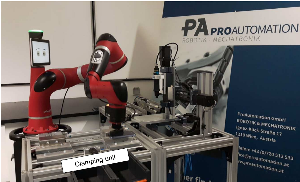
Figure 3: Robot places the smartphone into the clamping unit after heating it in the heating unit
