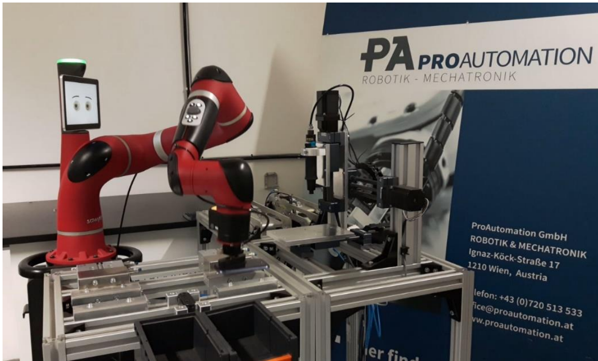
Figure 2: picture of demonstrator; bottom: clamping unit, right top: heating unit, right bottom: screwing unit, center: robot
