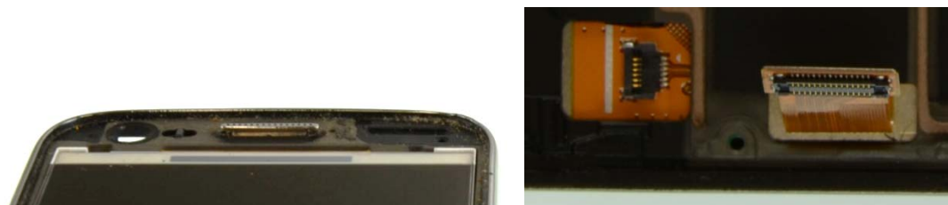
Figure 17: LCD line/row controller chip at upper end of LCD unit, left, and board connectors at LCD unit backside, right (Galaxy Ace 3)
