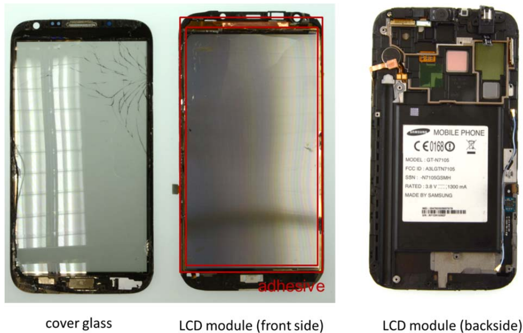
Figure 16: Display design with LCD module being glued into an internal frame, cover glass being glued to the edges of the LCD module frame (Galaxy Note 2)
