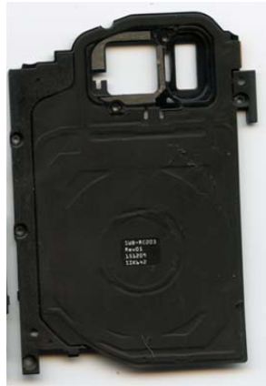
Figure 25: Integrated Qi-charging coil (Samsung Galaxy S7)
