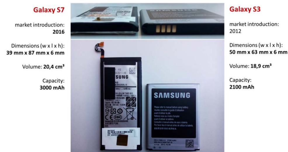
Figure 11: Comparison removable battery (Galaxy S3) and adhesive-fixed battery (Galaxy S7)
