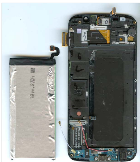
Figure 9: Battery fixed with adhesive strips (Galaxy S5)
