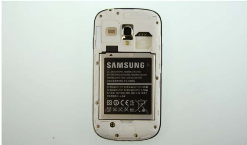
Figure 8: Battery removable without tools (Galaxy S3 mini)
