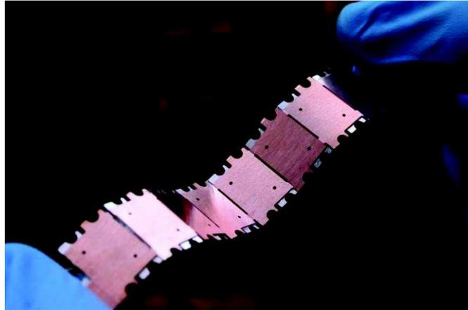
Figure 7: Mechanically flexible micro battery stripe made from segmented battery cells (© Fraunhofer IZM)
