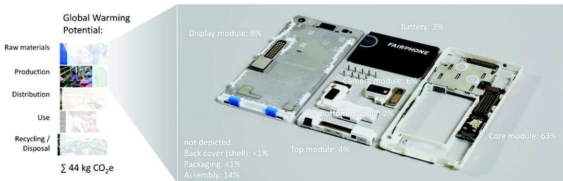
Figure 1: Modularity of the Fairphone 2 and the latter's carbon footprint
