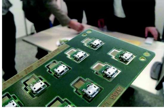
Figure 2: USB module for a mobile ICT device featuring embedding technology
