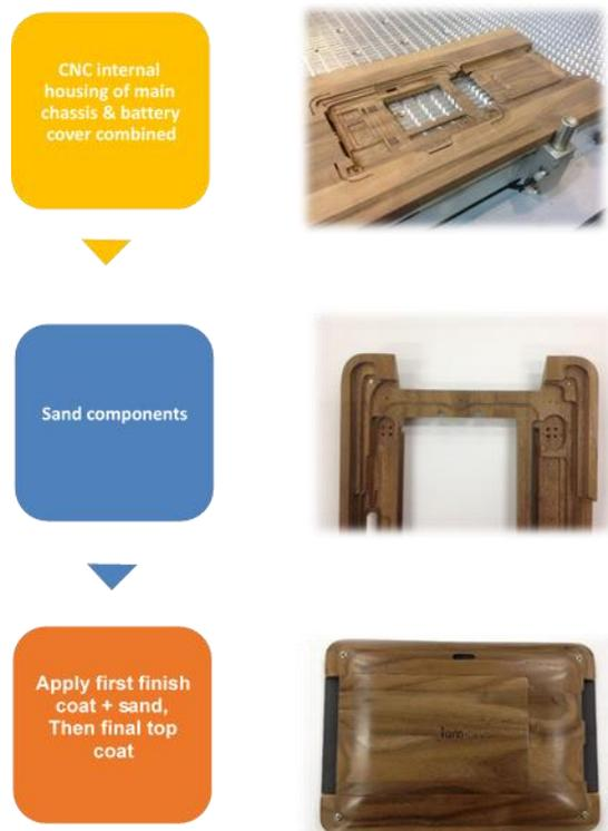
Fig. 12. Process Diagram (Part 2)
