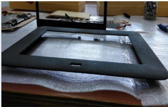
Fig. 14. Frame prototype 3D printed in plastics – front view
