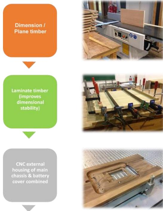
Fig. 11. Process Diagram (Part 1)
