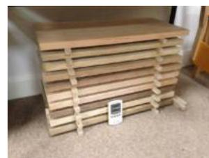
Fig. 13. Acclimatizing timber prior to machining
