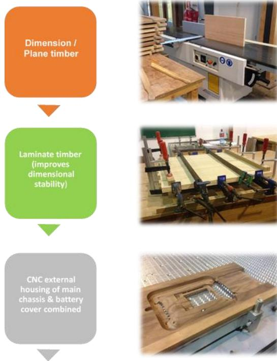
Fig. 11. Process Diagram (Part 1)
