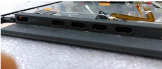
Fig. 15. Frame prototype 3D printed in plastics – connectors' slots view
