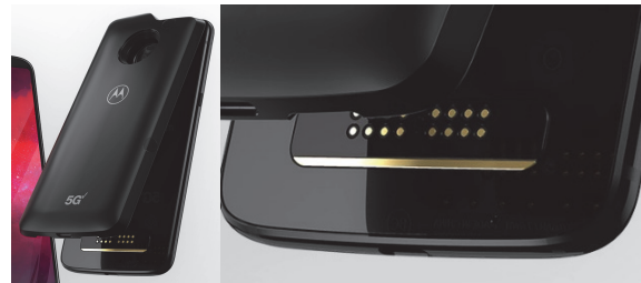
Figure 3: Moto 5G mod and close-up of the module connector [4]
